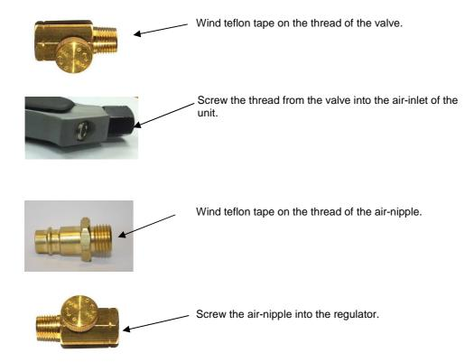
Norice: Basically we recommend to install a additional air pressure regulator with max. 6,5 bar (93 psi) and use the air-volume-control-valve for fine
